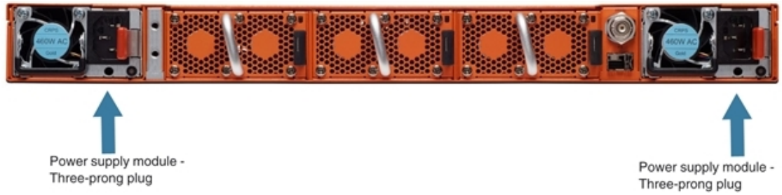
Figure 2 Connecting AC Power (GigaVUE-HC1)
